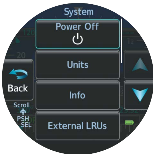
Battery Power-Off Menu
