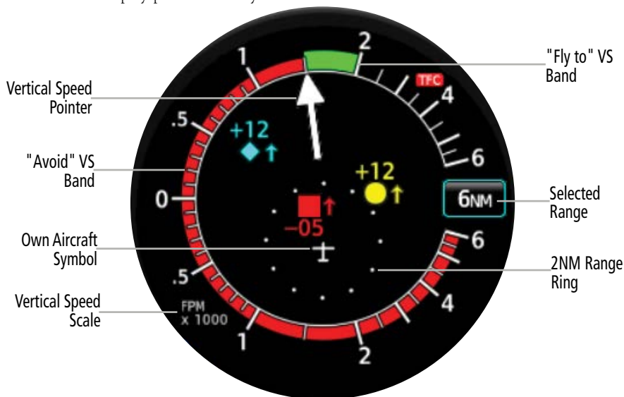
Instantaneous Vertical Speed Indicator
